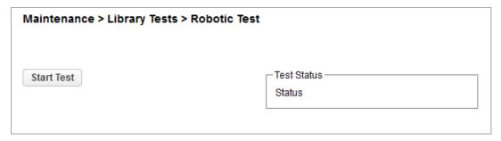
To run the robotic test, navigate to the Maintenance > Library Tests > Robotic Test screen, then click Start Test.
