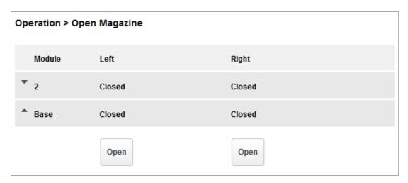
To unlock a magazine, click **Unlock** for the magazine and then click **Submit**. The library will release the lock. You can then open the door and pull the magazine out of the library to access the storage slots.
