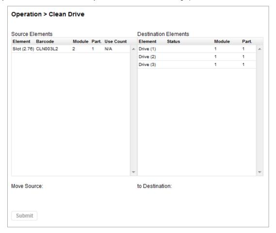
Select a cleaning cartridge from the Source Elements list. The library uses the barcode label to identify cleaning cartridges.
