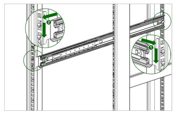
2. On the front of both rails in a square-hole rock, install a clip nut above the mounting bracket as shown, and for increased stability, install the retention inserts from the packet labeled **Retention Inserts**.
