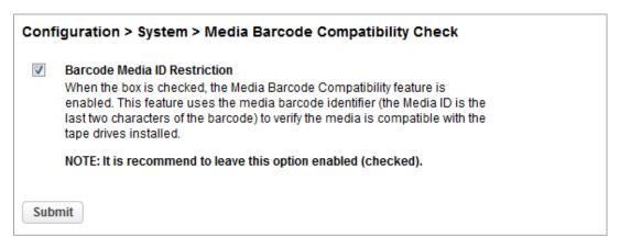
When **Barcode Media ID Restriction** is enabled, the library will only allow appropriate tape cartridges to be loaded into tape drives. The barcode media ID is the last two characters of the barcode. For example, an LTO-6 labeled cartridge will not be allowed to move into an LTO-4 tape drive.
