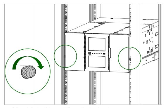
5. Repeat steps 2 through 4 to install the rest of the modules into the rack.
