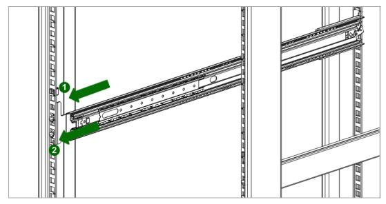
2. Slide the inner rails into the middle rails. Slide the module into the rack
