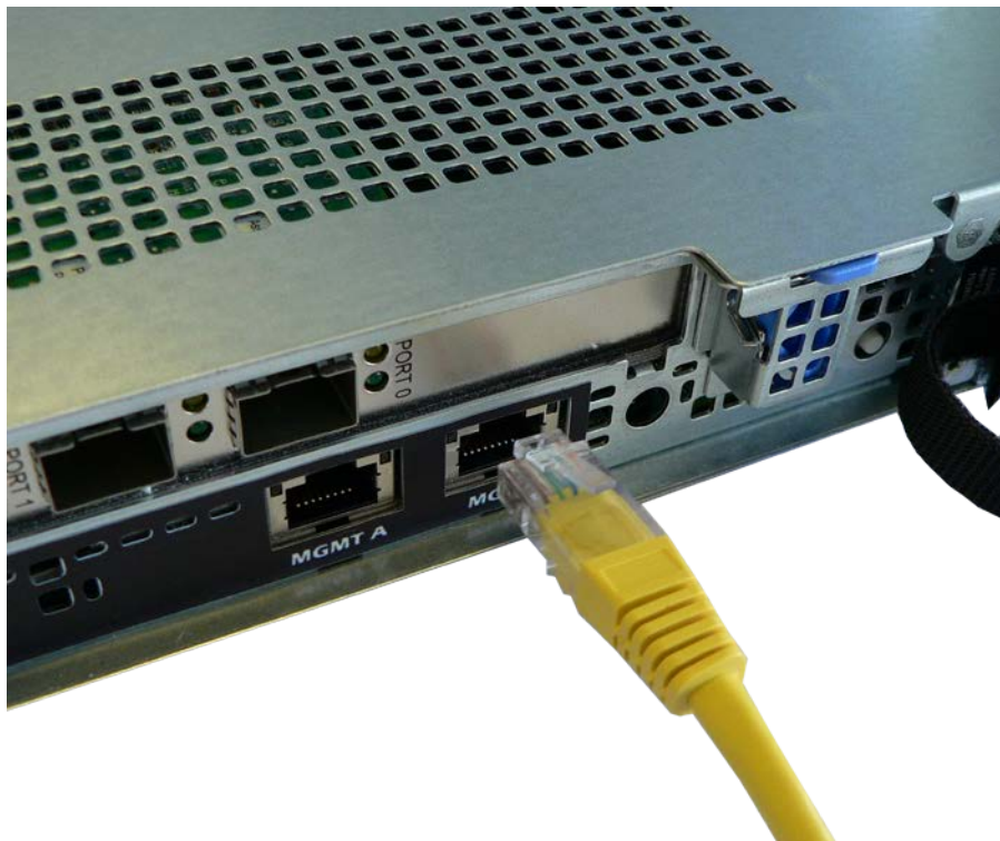
Rear Panel of the Bridge Showing Ethernet Cable Connections
