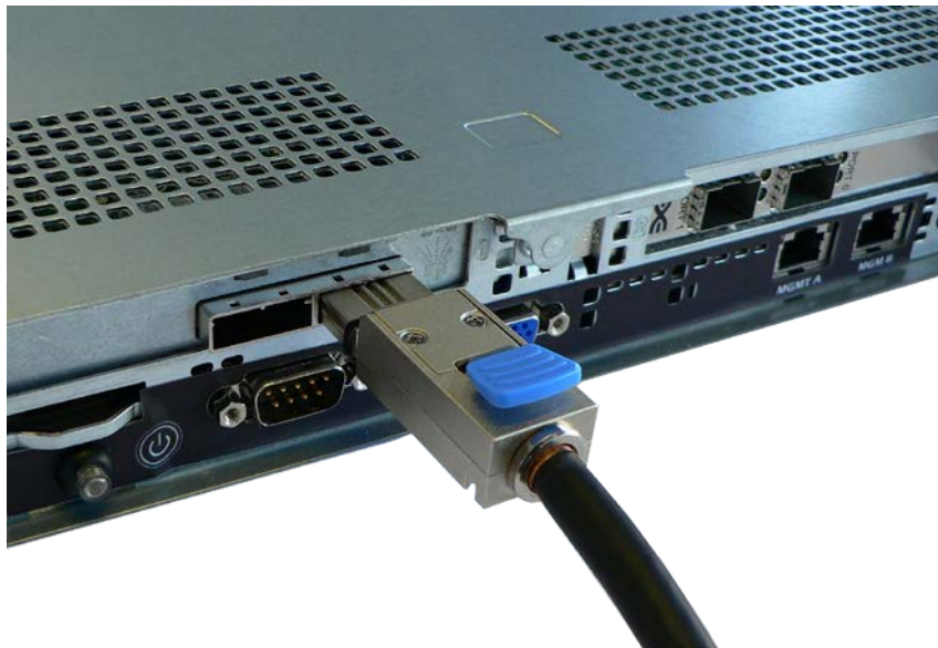
Connecting the SAS Cable to the Bridge SAS Port
