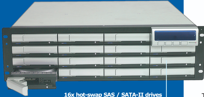
16x hot-swap SAS / SATA-II drives Capacities up to 16 Terabytes
